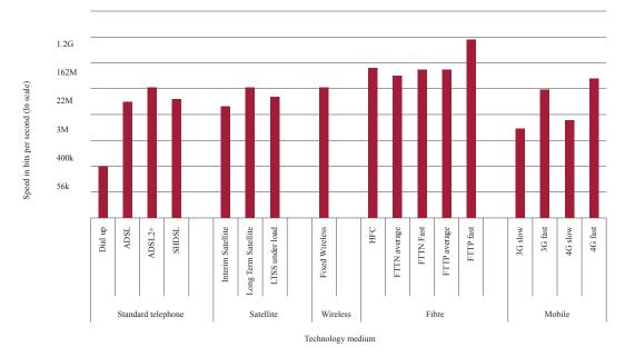
Figure 41: Download speeds by technology medium (bits per second, In scale)
