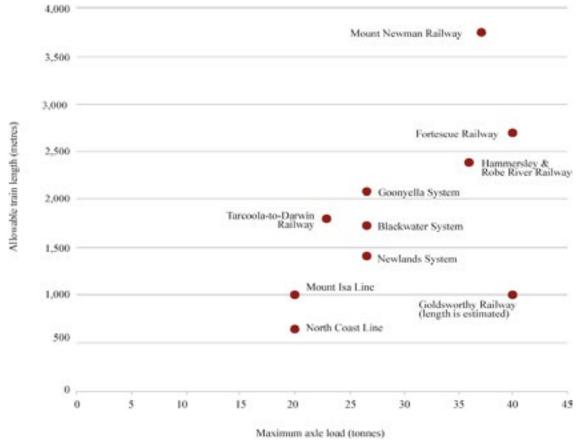
Figure 18: Allowable train length and maximum axle loads
